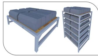
wooden pallet with iron sheet frame and steel legs from all sides reinforced with a horizontal crossbar between legs, and wood panels supported by locking screws fastening by passing through drilled hole in it.
