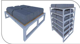
wooden pallet with iron sheet frame and legs from all sides reinforced with a horizontal crossbar between legs and column connected with frame and crossbar, and wood panels supported by locking screws fastening by passing through drilled hole in it.
